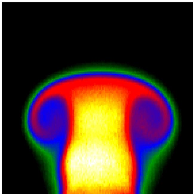
Fig. 3. Single-shot IR PLIF image of a vortex ring developing from a 6-mm tube. The jet fluid is 50% CO/50% Ar. The ambient gas is air. 12 mJ at  $2.35\ \mu\text{m}$  is used to excite the CO. The integration time is  $20\ \mu\text{s}$
