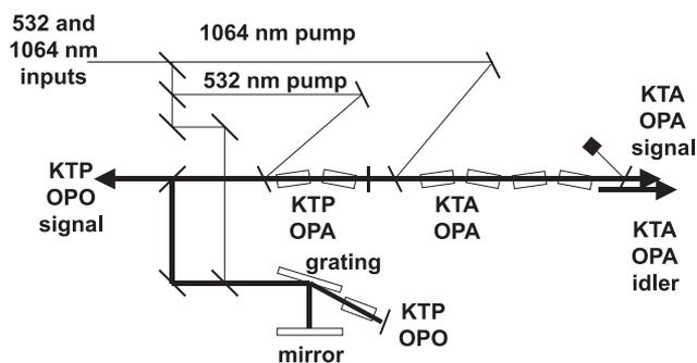
**Fig. 1.** Tunable infrared source consisting of modified Continuum Mirage 3000 OPO with KTA optical parametric amplifier stages added for increased conversion
