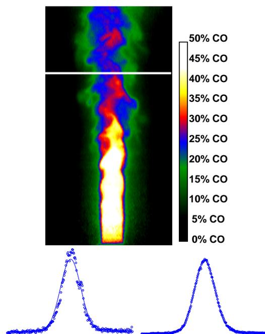
**Fig. 5.** Turbulent CO/Ar jet in CO/Ar/N<sub>2</sub> coflow. *Top:* Corrected single-shot instantaneous image. White line indicates  $x/D = 8$ . *Bottom:* normalized cuts at  $x/D = 8$  for instantaneous (*left*) and averaged (*right*) images are shown in comparison with the gaussian curve which best fits the averaged data. Integration time is 5  $\mu\text{s}$
