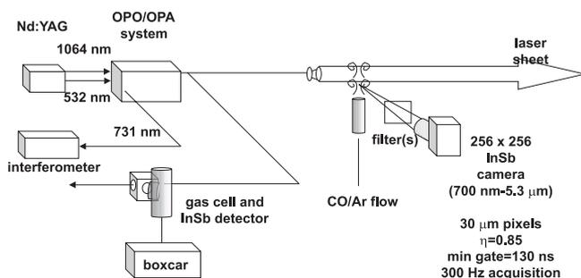
Fig. 2. Experimental setup for imaging experiments
