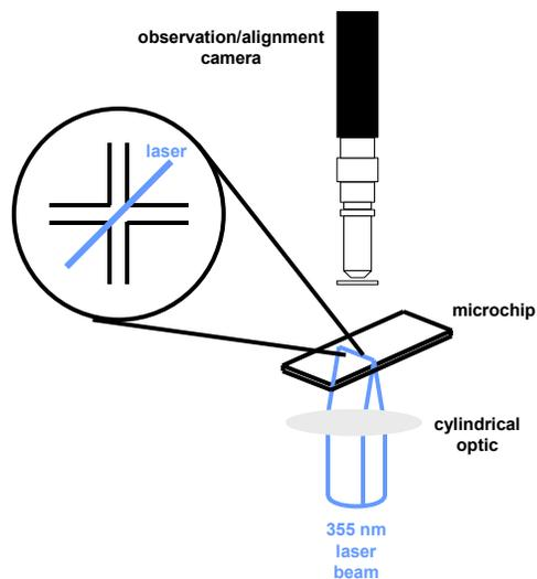
**Figure 2.** Beam-shaping optics for thin membrane polymerization.
