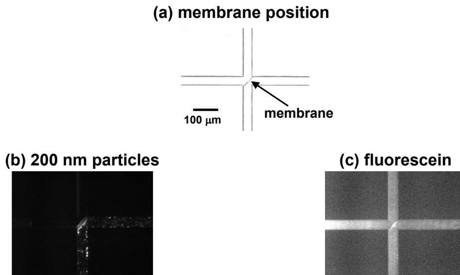
**Figure 3.** Images of selective diffusion across a 9  $\mu\text{m}$  porous polymer membrane: (a) white light image of membrane location; (b) fluorescence image of 200 nm fluorescent spheres, which do not diffuse across the membrane; (c) fluorescence signal from fluorescein, which does diffuse across the membrane.
