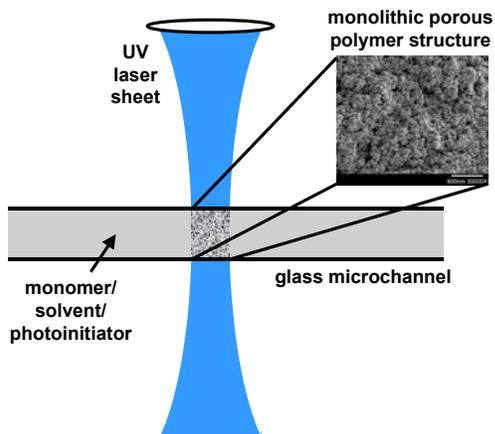
**Figure 1.** Phase-separation polymerization.
