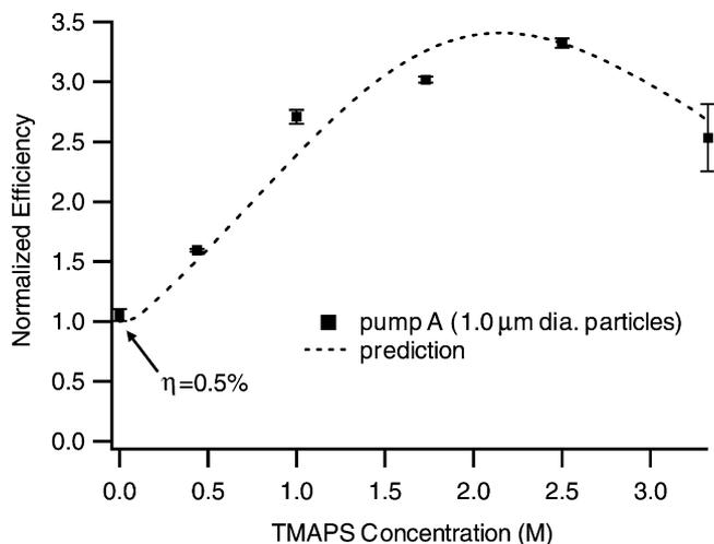
Fig. 6. Efficiency as a function of TMAPS concentration. Dashed line is a prediction Eq. (5) using experimental viscosity and conductivity data and a dielectric increment of  $52 \text{ M}^{-1}$ . The absolute value for the experimental  $\eta_0$  has been chosen to best match the prediction. Error bars indicate the standard deviation of the measured efficiencies at various voltages for each concentration.
