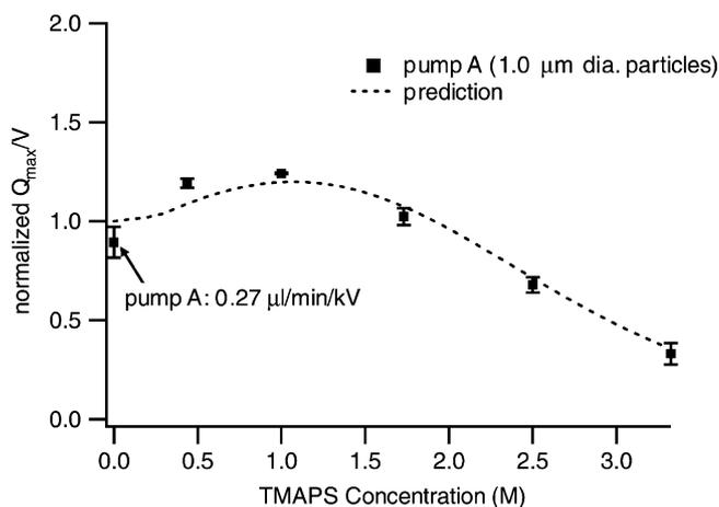
Fig. 5. Effect of TMAPS on  $Q_{\max}/V$ , measured at zero pressure. Dashed line indicates predicted  $Q_{\max}/V$  using experimental viscosity data and a dielectric increment of  $52 \text{ M}^{-1}$ . The absolute value for the experimental  $(Q_{\max}/V)_0$  has been chosen to best match the prediction. Error bars indicate the standard deviation of the linear fit of the flow rate vs. voltage curve at each concentration.
