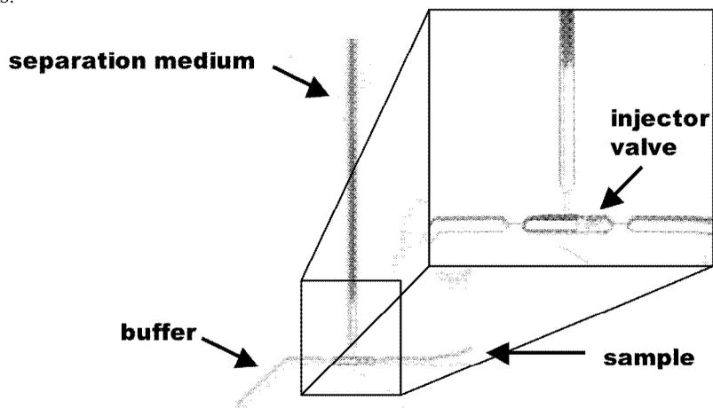
**Figure 2. Sample injection/separation geometry. Separation medium is patterned throughout separation column; valve element is localized at interface between sample and buffer lines.**
