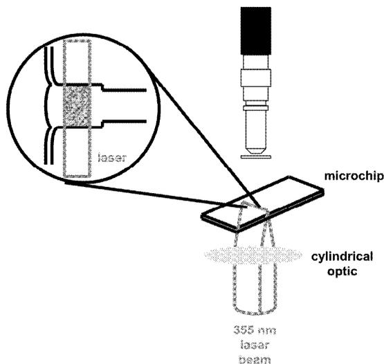
Figure 1. Projection lithographic setup used for patterning valve elements. Separation media requires less resolution, and is patterned using contact lithography.
