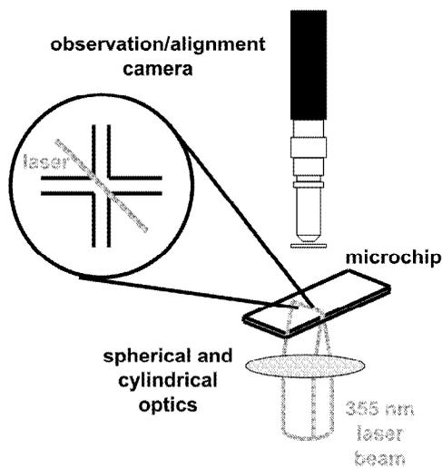
Figure 1. Laser-polymerization setup.
