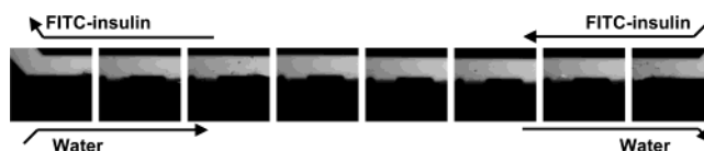
Figure 6. Lack of extraction of FITC-insulin (5700) in a counterflow dialysis configuration using the low MWCO membrane. The distance between the centers of the first and last images is 4.8 mm.
