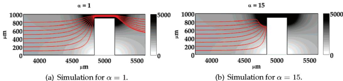
**Figure 2.** Simulated particle streamlines (red line) for high and low ac to dc ratios. Background color table corresponds to electric field magnitude. Simulation parameters:  $\phi_{\text{inlet}} = 50$  V, constriction ratio 10:1, particle radius  $1 \mu\text{m}$ .
