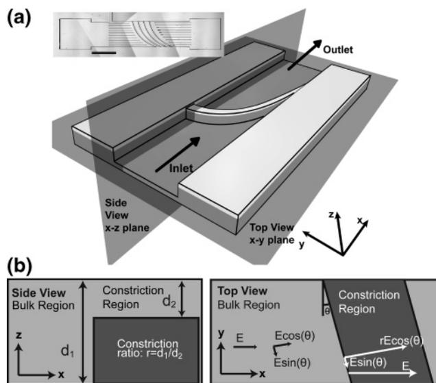
**Figure 1.** (a) 3D schematic of channel geometry. In (b), we define relevant geometric factors based on cross sections of the constriction region along the  $x$ - $y$  and  $x$ - $z$  planes.
