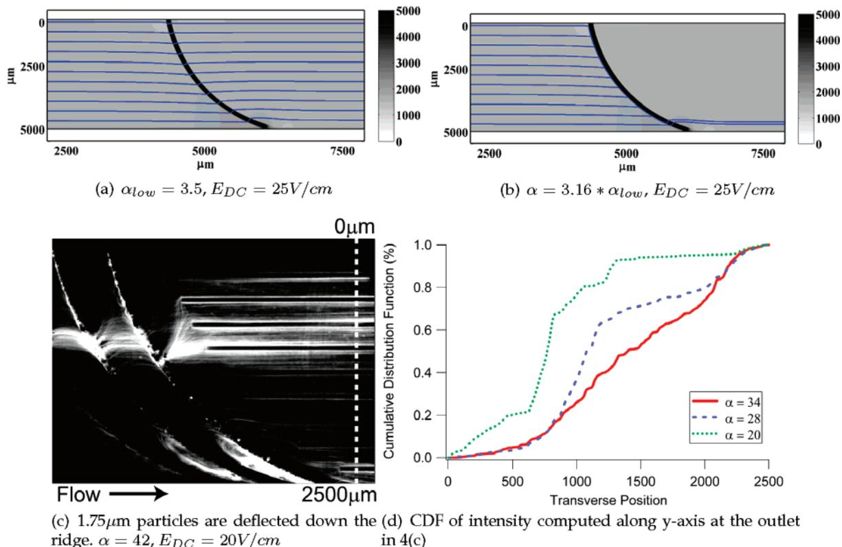
**Figure 4.** Varying the ac to dc ratio,  $\alpha$ , increases transverse ( $y$ -axis) deflection. Simulated particle pathlines in (a) show no net particle deflection at a low ac to dc ratio. (b) shows particle deflection tangent to a curved constriction in channel depth, transverse to the direction of flow for a high ac to dc ratio. Simulated particle radius of  $1\ \mu m$ . Electric field frequency is  $1\ kHz$ .
