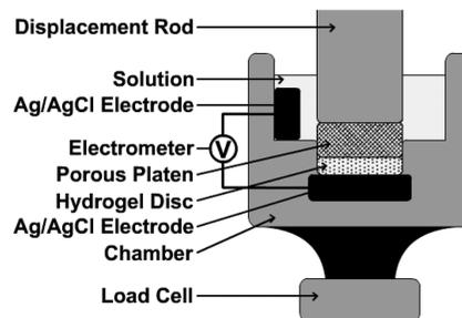
**Figure 1.** Testing apparatus for uniaxial compression in a radially confined geometry. Actuation of the displacement rod compresses the hydrogel disk. Fluid squeezed out of the hydrogel escapes through the porous polyethylene platen. Stress is registered by the load cell. Streaming potentials are measured by electrodes placed on opposite sides of the hydrogel disk.
