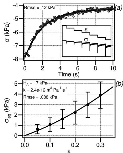
**Figure 2.** Stress relaxation tests performed on ionically cross-linked hydrogels. A series of step displacements produced stress responses that peaked and then decayed over time (a, inset). Each decay was fit by an exponential function (a), and the equilibrium stress followed a strain-stiffening constitutive relation (b). Bars are mean  $\pm$  standard deviation for  $n = 5$ . Rmse is the root mean squared error of the model fit.
