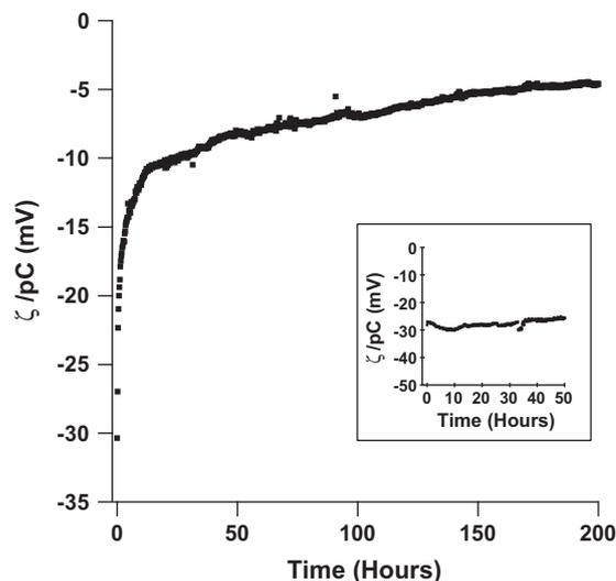
**Fig. 3.**  $\zeta$ -potential measurement in Zeonor at 1 atm over a time period of 200 h. The Zeonor data shown is an average of two replicates. The inset shows the electrokinetic potential in silica over a time period of 50 h for comparison. Data shown is  $\zeta$  normalized by  $pC = -\log(C)$  ( $C$  is the counterion concentration in M) as a function of time for a Zeonor substrate. 1 mM, pH 7 phosphate buffer was the working solution.
