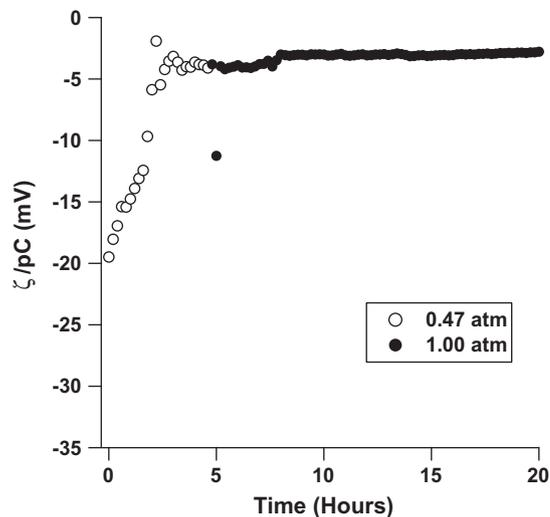
**Fig. 6.** The electrokinetic potential,  $\zeta$ , normalized by  $pC = -\log C$  ( $C$  is the counterion concentration in M) as a function of time for a Zeonor substrate. 1 mM, pH 7 phosphate buffer was the working solution. The experiment was initiated at 0.47 atm ambient pressure, and the pressure was raised to 1 atm after 5 h.
